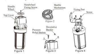
4 If you need to change the direction of water inlet and outlet, please take out the pressure relief button and decorative buckle on the top cover and adjust them to the opposite position (A and B holes are adjusted), and install them in place according to the hole position, as shown in Figure 3.
